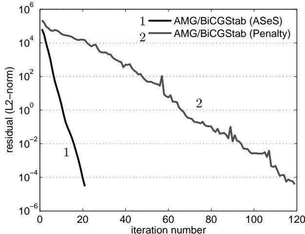
Figure 5: Residual reduction per iteration. ASeS resp. penalty approach and AMG-solver
