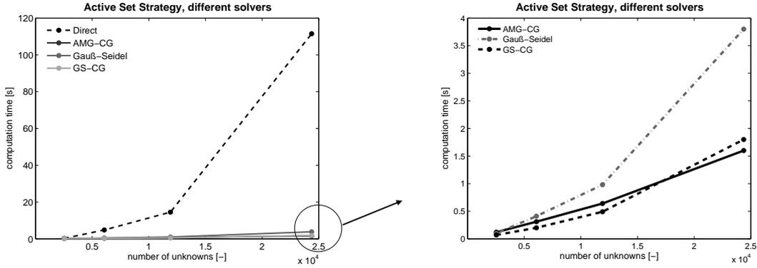
Figure 7: Averaged computation time per Newton step of direct and iterative solvers in connection with active set strategy
