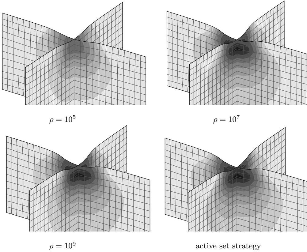
Figure 4: Deformed shape, loss in accuracy with decreasing penalty factor and active set strategy, von Mises equivalent stress  $\sigma_{seqv}$
