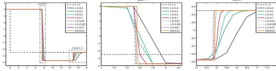
FIGURE 9. Macroscale approximation with  $\varepsilon = 10^{-5}$ ,  $\lambda = 4$ , zooms into the shock waves for different grid sizes.
