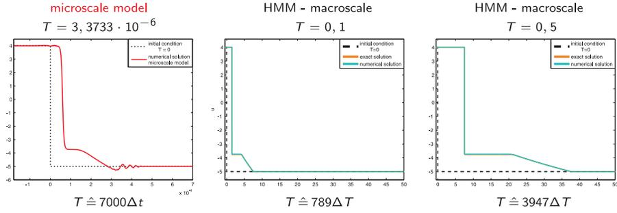
FIGURE 4. Shock-rarefaction solution for local regularization (10).
