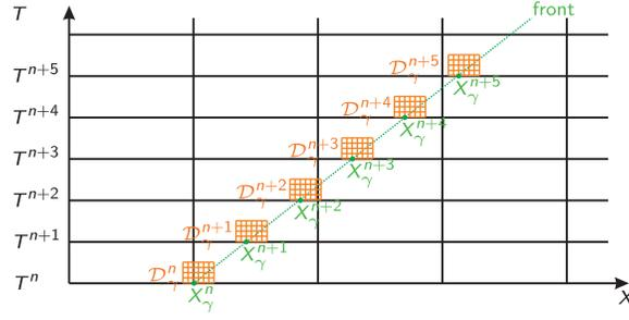
FIGURE 1. Macroscale computational domain  $\Omega_T$  and microscale computational domain  $\mathcal{D}_\gamma^n$  for a propagating front  $\gamma$  intersecting the macroscale time levels  $T^n$  in  $X_\gamma^n$ .
