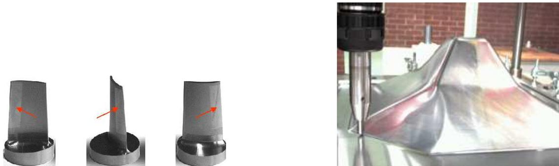
Figure 1: Deep-rolling process (©WZL, Aachen) and incremental sheet forming (©IBF, Aachen).
