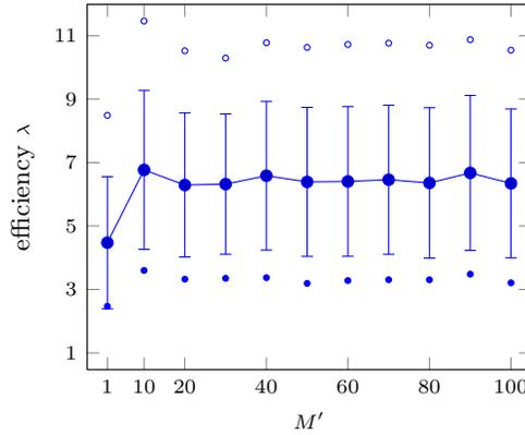
FIGURE 6.7. Error bar plot showing mean and standard deviation of error estimator efficiency over a sample of 20 random parameters for different values of  $M'$ . The dots indicate the minimum (●) and maximum (○) efficiency.
