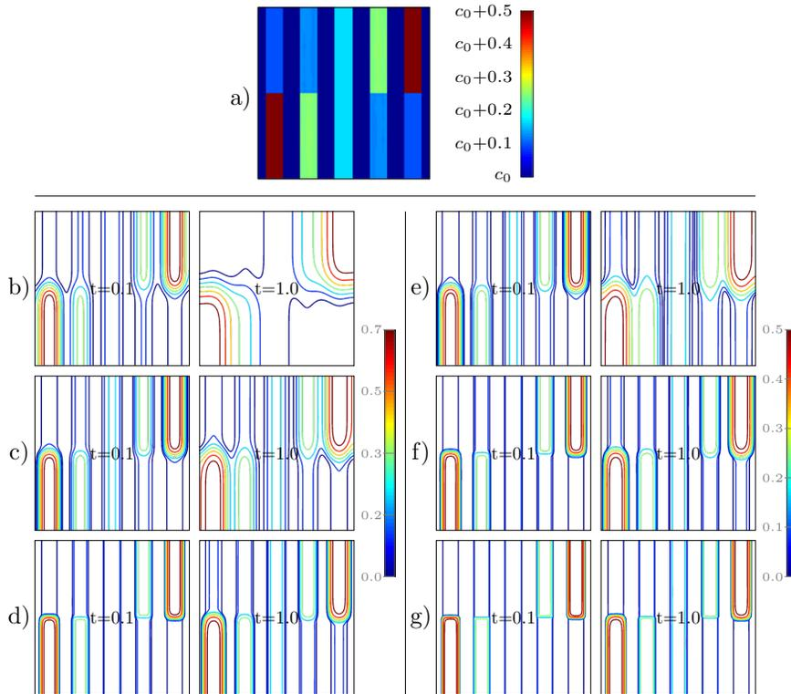
FIGURE 6.4. Plot a) depicts a color shading of the initial data. Below, isolines of reduced solutions are given at time instances  $t = 0.1$  and  $t = 1.0$  for different parameter vectors: b)  $\boldsymbol{\mu} = (1, 0.01, 0.2)$ , c)  $\boldsymbol{\mu} = (2, 0.01, 0.2)$ , d)  $\boldsymbol{\mu} = (4, 0.01, 0.2)$ , e)  $\boldsymbol{\mu} = (1, 0.01, 0.0)$ , f)  $\boldsymbol{\mu} = (2, 0.01, 0.0)$  and g)  $\boldsymbol{\mu} = (4, 0.01, 0.0)$ .
